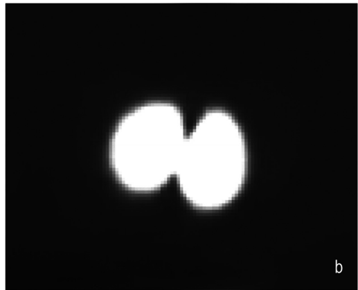
Figure 3. The fundamental (TEM 00 ) and higher order modes, obtained theoretically
